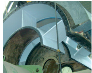
Lining of a classifier wheel shovel
